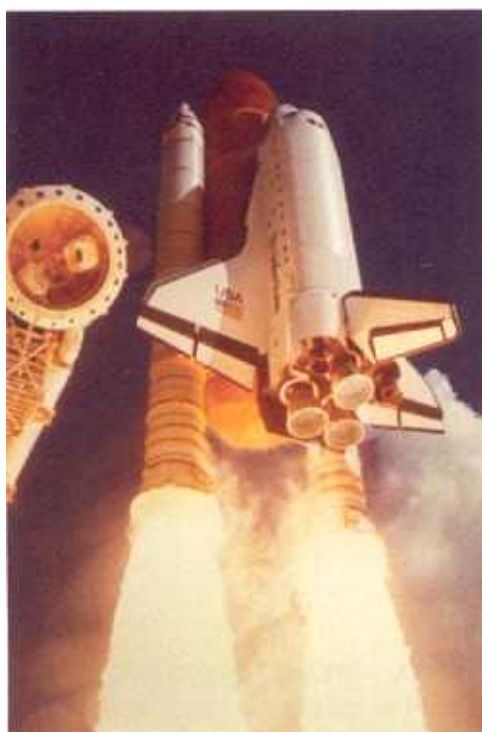
Figure 3.16 Energy released by the formation reaction between liquid hydrogen and liquid oxygen helps to propel the space shuttle into orbit.
