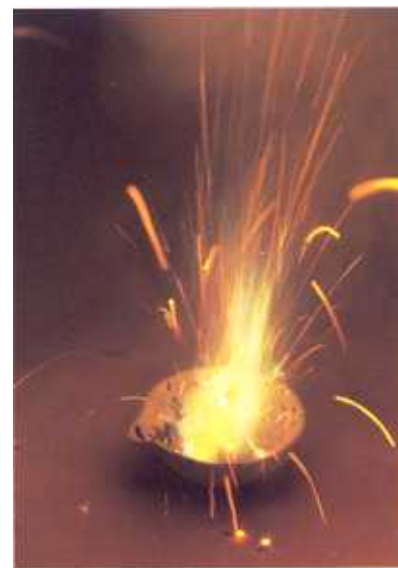
Figure 3.18 Decomposition reactions sometimes occur explosively. For example, when ammonium nitrate is heated, it explodes, forming dinitrogen monoxide and water.
