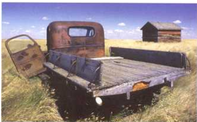
Figure 3.1 Iron in this truck reacted with water and oxygen to form rust.
